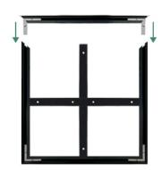
Insert last two corner connectors into remaining infinity frame, slide into connected one & tighten them with allen key & torx key.
